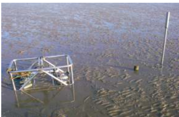
Side looking ADCP and Argus silt meter
